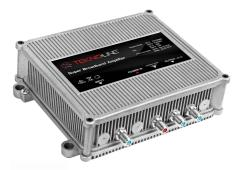
SBB (Super broadband) line amplifiers with return path. To be used as the final amplifier before wall outlets. Normally used to amplify the signals after an optical link. All adjustments are internally located under the die cast cover secured with safety screws to prevent unauthorised access. Packaging 1 pc.
